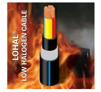
NHLSFR (Non Halogen) White Stripe cables are designed to reduce flame propagation and smoke in those instances where a fire may develop. By replacing the standard PVC with XLPE insulation and EVA bedding and outer sheath, no HCI gases will be liberated during the burning of the cables. (LOTOX®)
