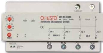
A Micro-processor controlled change over switch that automatically changes over to generator supply in the event of a power failure. A volt free signal is activated to engage the ignition circuit of the generator. On return of the main supply, the ACS will change back and de-activate the generator ignition signal.
